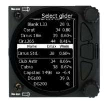
You can modify the polar by changing coefficients **a**, **b** and **c**. A polar is defined as a quadratic equation with the parameters a, b, and c.
