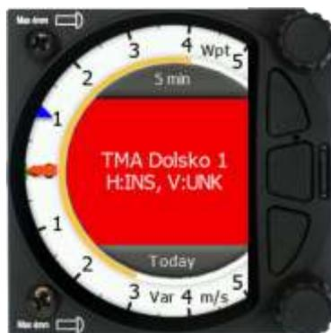
The first row is a name of the airspace. You can terminate a warning for 5 minutes by pressing an upper button or lower button, which will cancel it for today.
