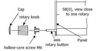
Remove the two rotary knob caps with a knife or flat screw driver, then hold each knob and unscrew it. Remove the remaining two screws and the two M6 threaded nuts. Install the S8x/S10x into the panel and screw back all screws, nuts and knobs. Ensure that between the knobs and the panel there is sufficient space so that the button can be pushed.
