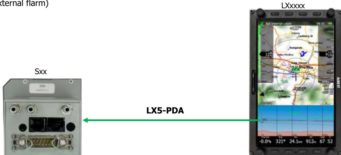
This configuration is used for example when using your Sxx vario together with LXxxxx and Flarm device (e.g. FlarmMouse). LX5-PDA is connected to **PDA port** and **external flarm** to the **GPS port**.
