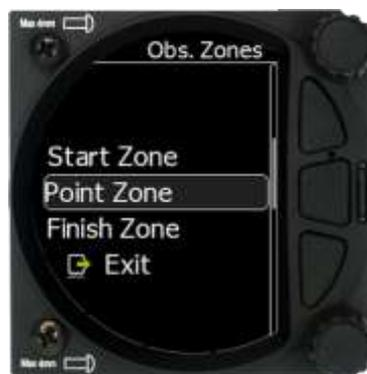
The Start, Waypoint and Finish zone can be configured separately although the setup is very similar.
