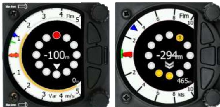
*The warnings continue as long as FLARM calculates a threat of collision. The warning level may decline or be cancelled, depending upon the prediction. The warnings are selective; they are only issued if the calculation reveals a high probability of collision in the near future.*
