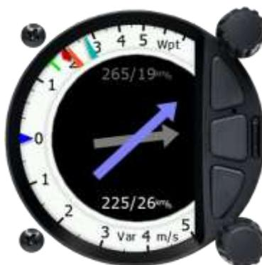
When using **HAWK** option, default average time for wind is set to 30 seconds. User can modify it in Vario parameters. If **HAWK** option is not used, averaging time is fixed to three minutes. To learn more about **HAWK** see chapter 7.
