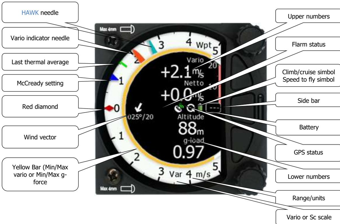
The Vario **Needle** can display: the Vario, Netto, Relative or Speed to fly value (Setup->Hardware->Indicator). The scale can be chosen in the range of +/-5 +/-10 or +/-20. The cursor style can be thin, medium or thick. It can be linear or non-linear (setup->graphics->indicator). Within the software the range can be set to m/s, kts, km/h, mph or fpm (in Setup, Units, Vertical speed).
