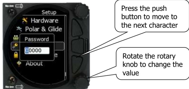
Once the required value is selected, press the lower push button to move to the next character selection. To move back to the previous character, press the upper push button. When you have finished editing, press the Enter key – the lower rotary button. A short press of the middle push button exits from the edited field (“control”).
