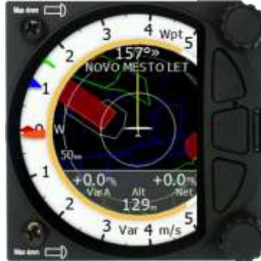
The first page shows a line to a selected waypoint, the name of the selected waypoint at the top of the screen and the relative bearing with chevrons indicating the direction to turn towards the selected waypoint.
