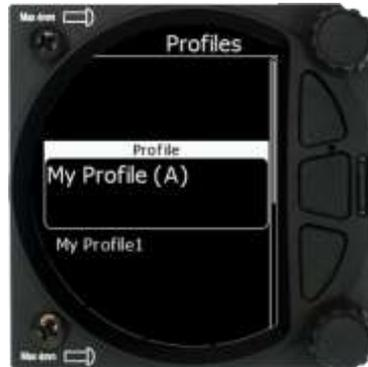
With the lower rotary knob, a pilot can scroll between different profiles that are stored within the internal storage of the S vario. Please note that the profiles are not stored on the SD card.
