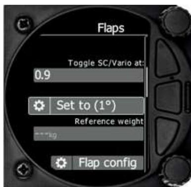
When all flap positions are set, a green dot will be displayed with current flap position. If flap labels are not set yet, press **EDIT** to name the labels. Flap labels must be entered with increasing speed range. It is recommended that flaps labels are set together with the speed range in the Polar and Glider setup. It is also possible to toggle between cruise and climb mode using the flap sensor.
