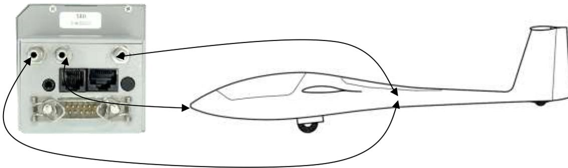
If the unit is to be configured for pneumatic TE compensation using a TE tube, then the connections are:
