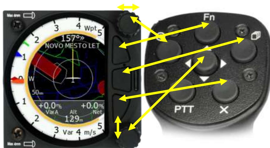
The remote stick is also connected to the CAN bus. On the S8x/S10x a special menu is provided to register the remote stick. The device must be registered in case of two-seat device; it is possible to have two remote sticks, one registered on the front and another on the rear device. Older types of remote sticks having wired SC button, which can be connected to one of the vario inputs. Newer type has not any more this cable, the function of the front SC button is permanently set to SC toggle.
