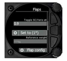
When all flap positions are set, a green dot will be displayed with current flap position. If flap labels are not set yet, press **EDIT** to name the labels. Flap labels must be entered with increasing speed range. It is recommended that flaps labels are set together with the speed range in the Polar and Glider setup. It is also possible to toggle between cruise and climb mode using the flap sensor.
