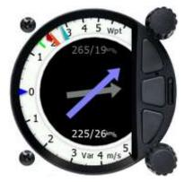
The two-needle approach helps to optimize the thermaling performance by comparing the real climb rate of the red needle ("TEK vario") to the potential climb rate of the blue needle ("Hawk vario"). For example, if the pilot flies with a large sideslip angle, the difference between the two needles can be minimized by flying with a smaller sideslip angle. The red needle will approach the blue needle: the real climb rate has become larger.
