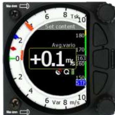
The navigation boxes in this second task page can be changed using the Quick Access menu and selecting **navbox**.
