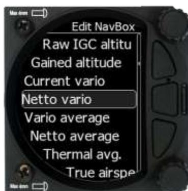
Select the required navbox and then save this with a short press of the lower rotary knob. Repeat the process for any other navbox that needs to be changed.
