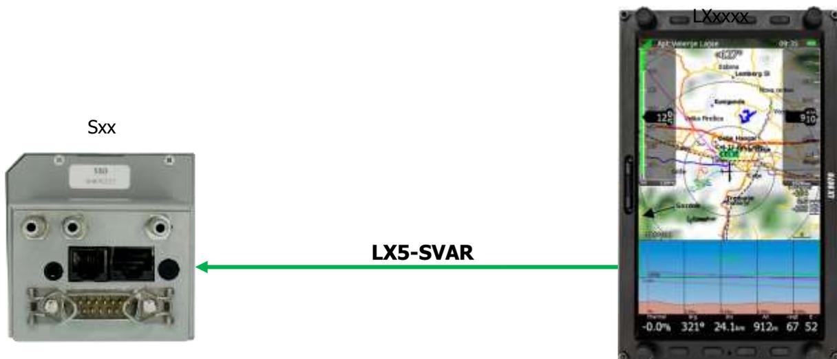
This configuration is used for example when using your Sxx vario together with Oudie and LXxxxx. **LX5-SVAR** is connected to **GPS port** and **CC-NP-LOUDIE** cable to **PDA port**.
