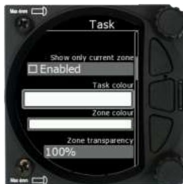
With this dialogue you can change the colour of the task line and turn point zone and modify the zone transparency and Zone line width.
