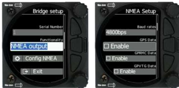
NMEA output is used to transmit NMEA sentences. You can select desired NMEA sentences and define the baud rate at which they will be transmitted.
