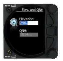
The instrument will offer elevation over standard pressure level QNE. Use the knob to fine-tune the elevation.
