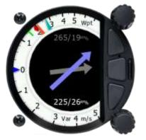
When using HAWK option, default average time for wind is set to 30 seconds. User can modify it in Vario parameters. If HAWK option is not used, averaging time is fixed to three minutes. To learn more about HAWK see chapter 7.
