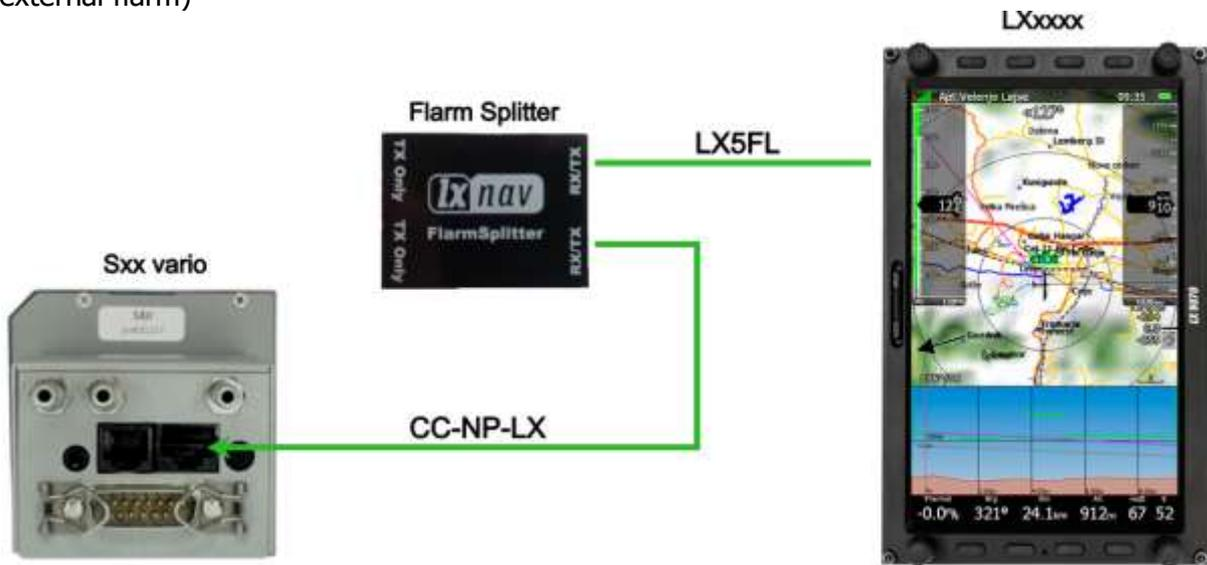
Option 2: From Sxxx **GPS port** to LXxxxx on a **5pin** Connector using **LX5-SVAR**. (PDA port is free to connect Oudie or other PDA device)
