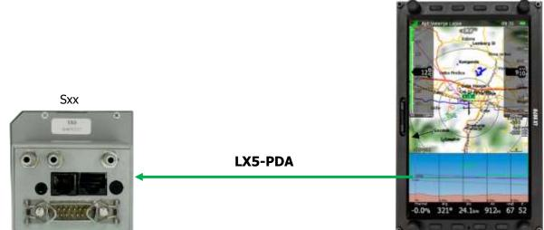
This configuration is used for example when using your Sxx vario together with LXxxxx and Flarm device (e.g. FlarmMouse). LX5-PDA is connected to **PDA port** and **external flarm** to the **GPS port**.
