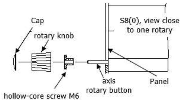
Remove the two rotary knob caps with a knife or flat screw driver, then hold each knob and unscrew it. Remove the remaining two screws and the two M6 threaded nuts. Install the S8x/S10x into the panel and screw back all screws, nuts and knobs. Ensure that between the knobs and the panel there is sufficient space so that the button can be pushed.
