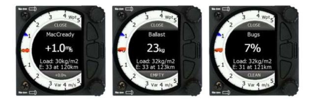
Rotate the lower knob to modify any setting. Next check the safety altitude (height above destination, arrival altitude) setting.
