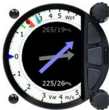
The two-needle approach helps to optimize the thermaling performance by comparing the real climb rate of the red needle ("TEK vario") to the potential climb rate of the blue needle ("Hawk vario"). For example, if the pilot flies with a large sideslip angle, the difference between the two needles can be minimized by flying with a smaller sideslip angle. The red needle will approach the blue needle: the real climb rate has become larger.
