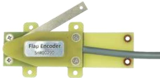
The Flap sensor must be connected to the CAN bus through a CAN bus (Y) splitter. Any remaining ports on the Y CAN splitter must be terminated with a CAN terminator.
