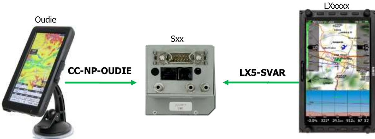
Option 3: From Sxxx **PDA** to LXxxxx on **5pin** connector (to the **GPS** port can be connected external flarm)
