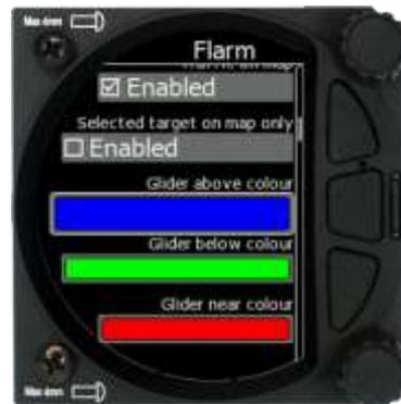
In this menu you can choose to show FLARM traffic on the map, select target on map only, change glider colours and adjust the FLARM object timeout and graphical settings.
