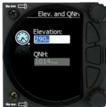
The user must set either the Elevation or the QNH with the lower rotary button. After pressing the lower rotary button, the user can switch between the Elevation and QNH dialogues. As soon as the settings are set the middle button must be pressed to proceed.
