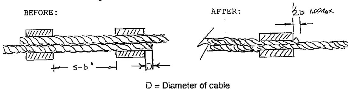
3. Place the ferrule (and cable) between the dies, vertically and centrally.
