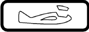
OPEN and/or EMERGENCY JETTISONING of rear canopy: Move red levers LH and RH on canopy frame backwards
