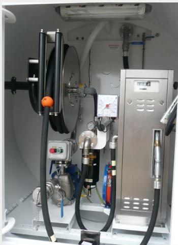
TANKS FITTED WITH HIGH QUALITY FUEL DISPENSING EQUIPMENT FOR MAXIMUM EFFICIENCY AND RELIABILITY
